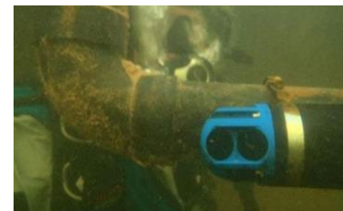
Acoustic sensor for continuous data on Colorado River (calibrated by conventional samples)
